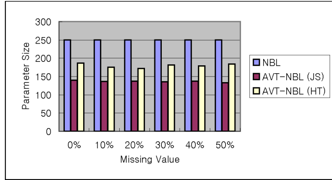
Figure 4.7 The size (as measured by the number of parameters) of the Standard Naive Bayes Learner (NBL) compared with that of AVT-NBL on AGARICUS-LEPIOTA data. HT stands for human-supplied AVT. JS denotes AVT constructed by AVT-Learner using Jensen-Shannon divergence.
